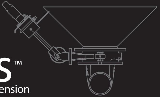
BTI's new EasyAccess™ Multi-Angle Neck Extension allows for effortless operation of all BTI Butterfly Valves. No more crawling under tank trailers in messy situations. No more back injuries and workman compensation claims due to awkward angles and burns from air supply lines that can reach 350°F.
