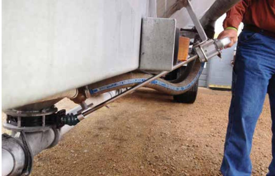
**(a)** The EasyAccess™ Multi-Angle Neck Extension consists of a universal joint securely fastened to the stem of the butterfly valve. **(b)** A rubber boot over the u-joint seals contamination out of the joint and retains lubrication. The other half of
