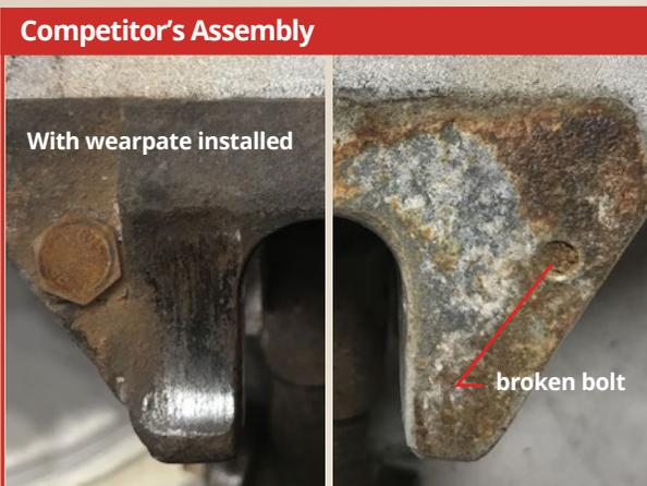
Corrosion builds up between the lid and the bolts making the replaceable wearplate *non-replaceable*. When it is time to replace the wearplates the heads of the bolts break off causing major time and, in some cases, total lid replacement.
