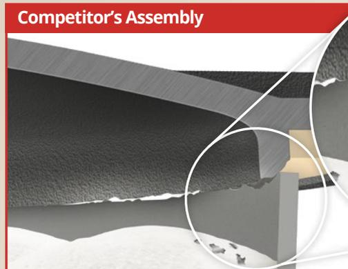
Competitor's lid with metal alignment lip causes chipping of collar and aligner allowing metal to end up in the load.
